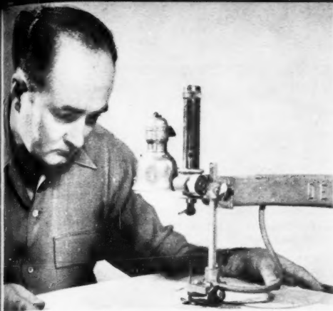
Cutting the printing aperture in the center of the plywood top. All the edges should be sanded.
